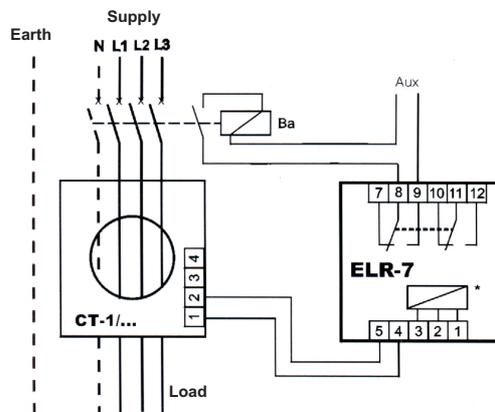
Wiring diagram for MCCB with shunt trip and energized end relay to the trip (FAIL SAFE OFF) for using de-energized (FAIL SAFE ON) connecto the BA the terminals 7 - 8 (contact NO in no tripped condition)
