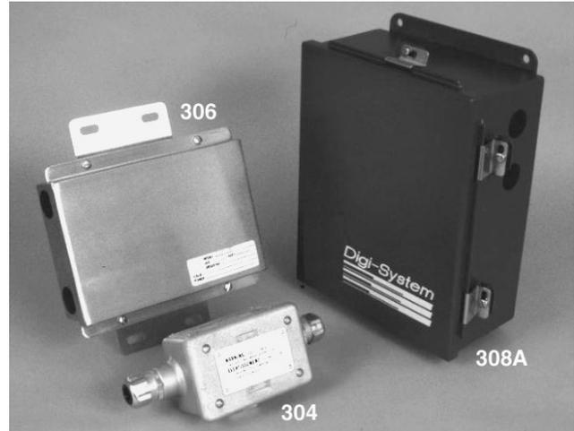
304 Extension Boxes are used whenever transducer cables are not long enough to reach the summing unit or system instrumentation. The internal terminal block or connection provides for either a four wire or six wire (remote sensing) hookup. A range of metallic enclosures are available for washdown, corrosive, and electrical hazard applications.
