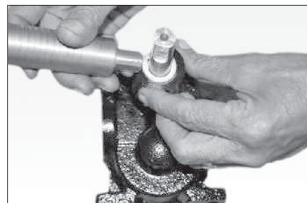
Fig.11. Installing gasket using pipe assembly
