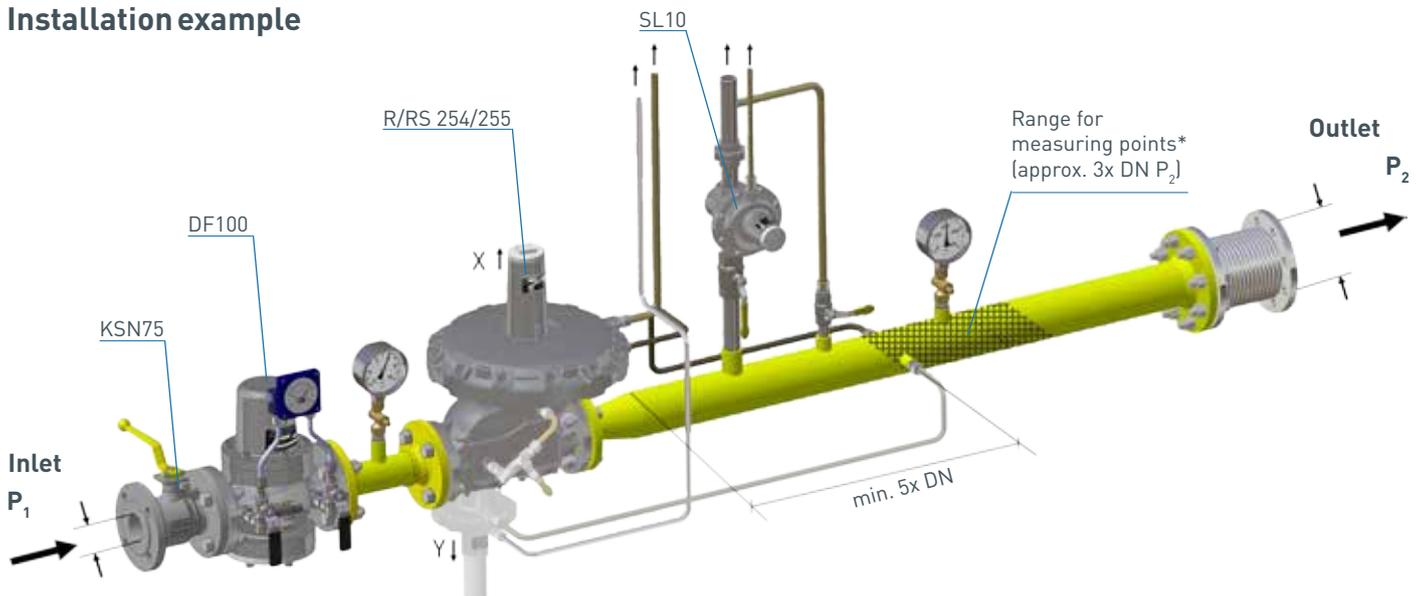
\*) Recommended max. velocity at the measurement line port 25 m/s
