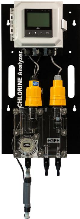
The GF 4630 Free Chlorine Analyzer System is an integrated all-in-one system designed to measure free chlorine. The 3-4630 Free Chlorine Analyzer with pH sensor is used to accurately calculate free chlorine in applications that have varying pH values ( $\pm 0.20$  pH units).
