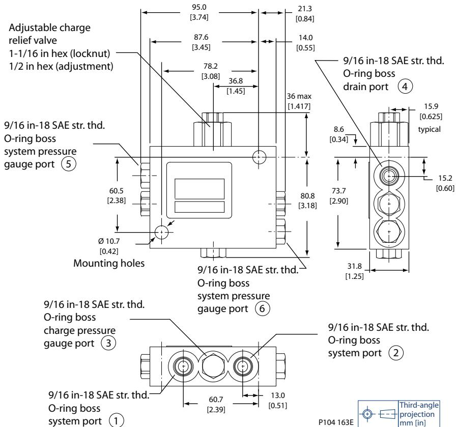
Mount the loop flushing valve on any convenient flat surface that provides adequate support around the two mounting holes. Ensure the surfaces under the mounting bolts form a flat plane.
