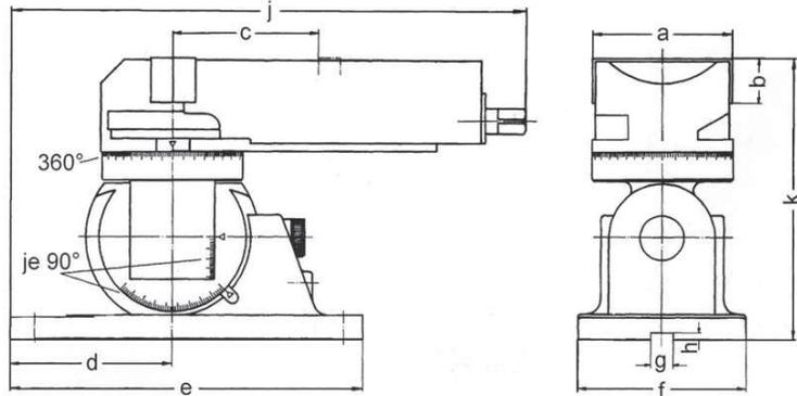
Clamping force: max. 10 kN at approx. tightening torque 30 Nm
