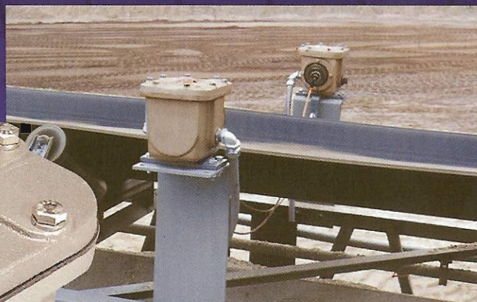
VIEW OF CONVEYOR SHOWING UNIT MOUNTED WITH CABLE UNDERNEATH (2 REQUIRED)
