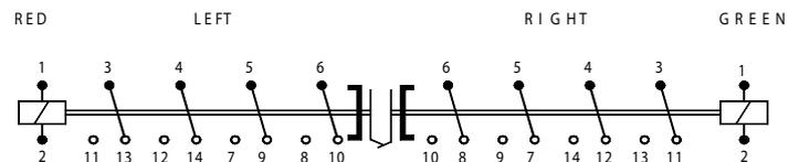
Please note the relay will leave production in open state (with open armature at the left side, flag is green) with all contacts in the position shown in the connection diagram. Due to severe shocks far exceeding maximum levels mentioned in IEC 61373 (Category I, Class B, Body mounted), it can happen the left armature closes and stay closed. Therefore after installation all relays must be checked on correct state of the contacts and activate both coils 10 times alternately for correct operation.
