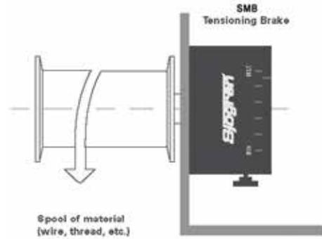
Usual set-up for tensioning wire, film, etc. on pay-off.
