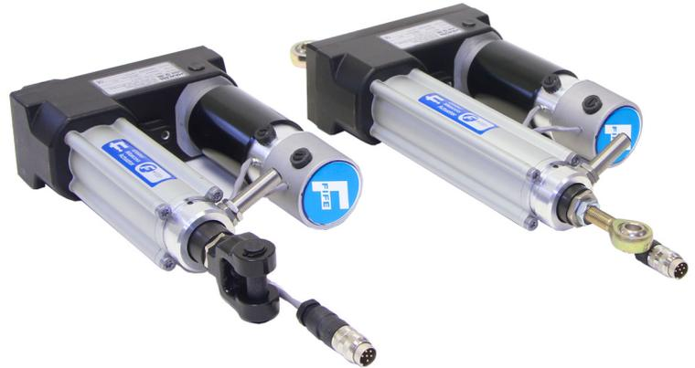
Ball screw and nut design provides low-friction, efficient operation and eliminates the typical end of stroke sticking and need for actuator limit switches. Compatible with all of Fife's controllers, this actuator is widely used for steering guides, displacement guides, positioner assemblies, slaving, chasing applications and unwind/rewind applications.
