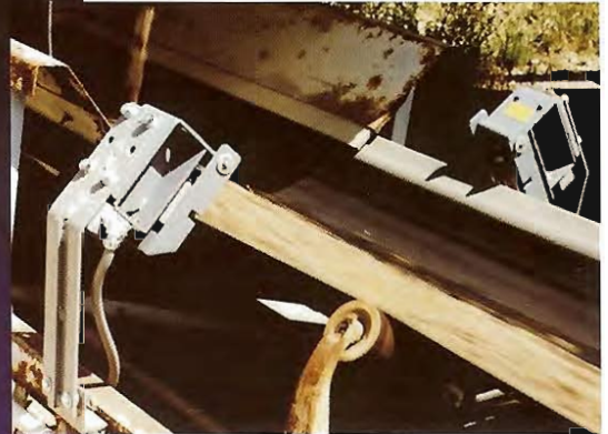
Shown are two BA units protecting a valuable conveyor belt from damage due to belt misalignment or run-off at an aggregate facility
