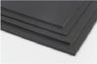
Eccosorb GDS is a thin, flexible, high-loss, magnetically loaded, electrically non-conductive silicone rubber sheet. It is designed for the frequency range from 6 GHz and above. The material is impervious to moisture and can be subjected to high altitudes, with no adverse effects. Being a silicone based absorber, it has low outgassing properties for space applications.
