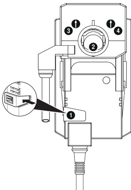
**Note:** Perform settings on the auxiliary switch only in deenergised state.
