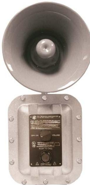
GAI-TRONICS Model 400-001 and 400-002NS RigCom Stations are a common-talk communication system designed for hazardous and harsh environments. The system is simple to use with push-to-talk, release-to-listen operation. The station can also be configured for hands-free operation where the speaker is always in listen mode. The RigCom station consists of an explosion-proof case, which houses the electronics, and an explosion-proof loudspeaker that also functions as the microphone.
