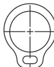
Lug Design For Sizes SH-12 thru SH-23
