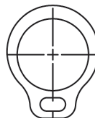
Lug Design For Sizes SH-12 thru SH-23
