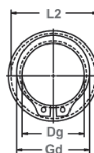
Clearance Diameter & Gaging Diameter Released in Groove.
