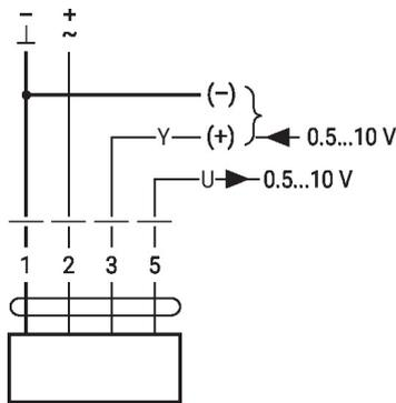
Override control (frost protection circuit)
